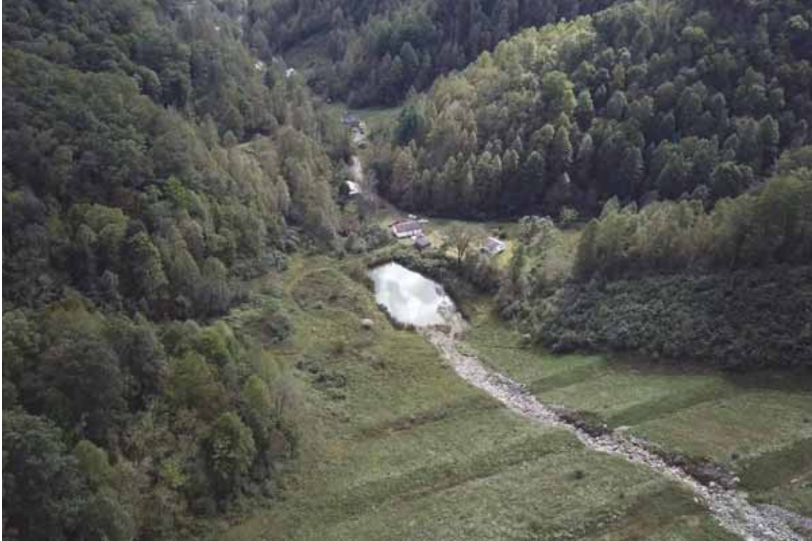
One of the mine's valley fills. The rocks replace a buried stream and water collects in a sediment pond below, feeding into a stream that runs alongside a row of homes, all of which rely on private wells.
