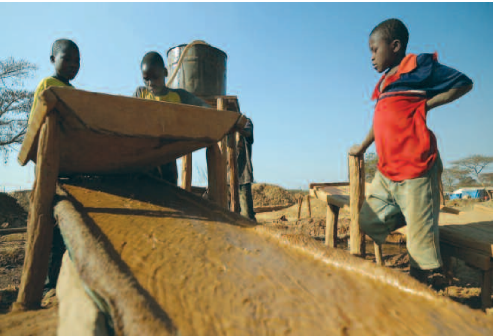
Two 13-year-old boys and one 15-year-old boy pour crushed gold ore over a sisal sack to concentrate the particles of gold at a processing site in Mbeya Region.
