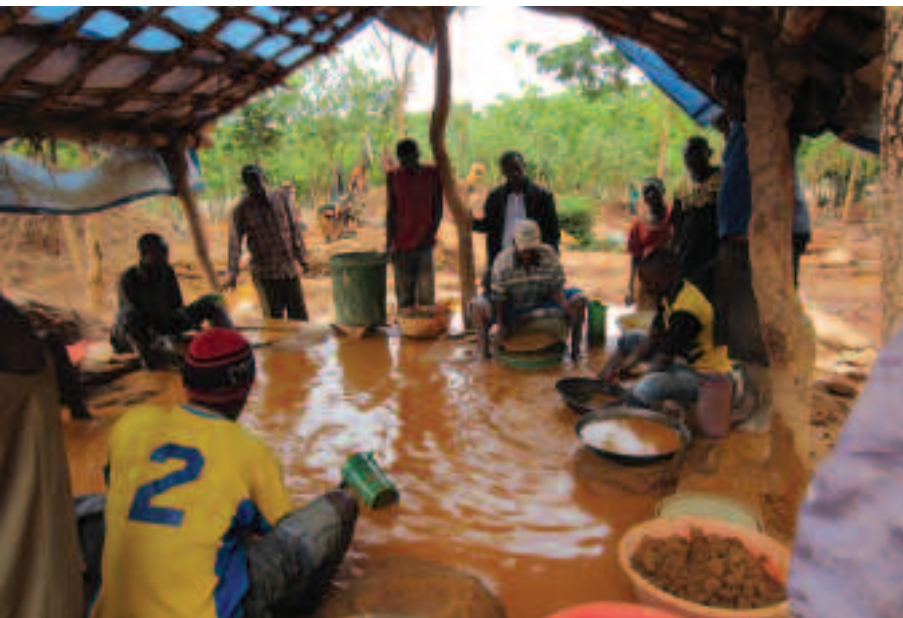
Miners mixing mercury and ground gold ore in an amalgamation pond in Geita Region.
