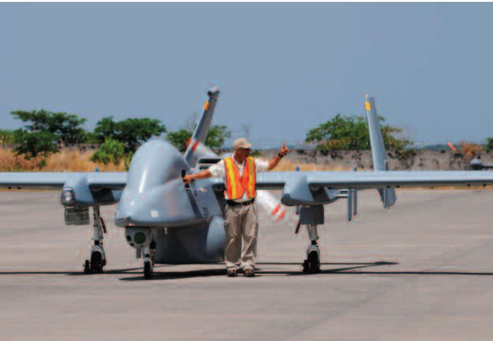
An Israeli-made Heron UCAV (unmanned combat aerial vehicle). A gimbal camera is seen underneath the aircraft's nose.
