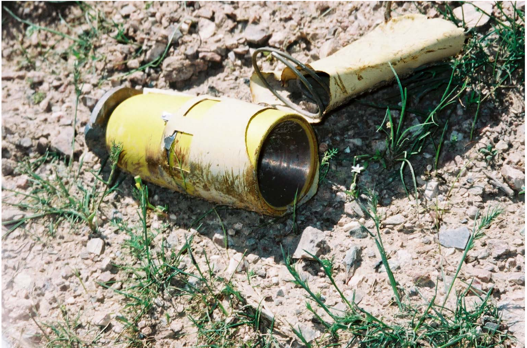
Two BLUs lie in a field in Shidai near Herat. The left bomblet is unexploded. The shaped charge, an anti-armor concave cone, is visible at its right end, and the exterior canister has slipped to expose its antipersonnel fragmentary core. On the right is the flattened canister of a bomblet and the spring that pushes out the parachute and arms the bomblet. © Bonnie Docherty / Human Rights Watch, 2002.
